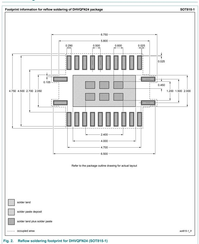
plastic, leadless dual in-line compatible thermal enhanced very thin quad flat package; 24 terminals; 0.5 mm pitch; 3.5 mm x 5.5 mm x 0.85 mm body
